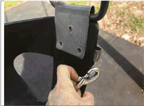
Missing link to chain safety belt to
