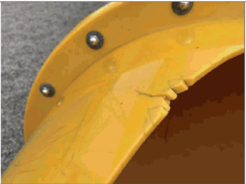
Tube slide broken/sharp.
