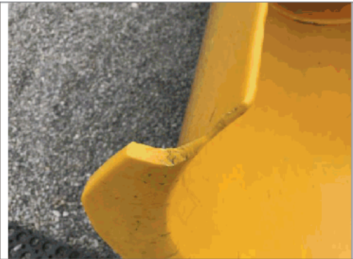
Tube slide broken/sharp.
