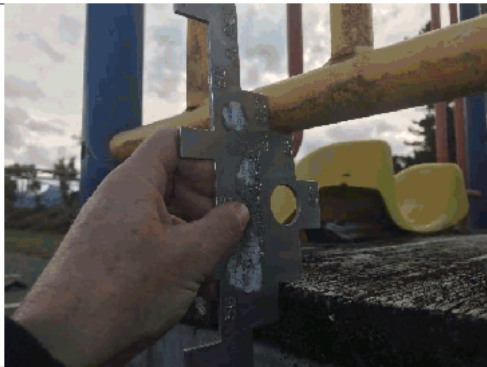
Head entrapment under barrier on module
