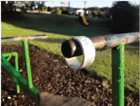
Handles fail ring gauge test (should not pass through ring)
