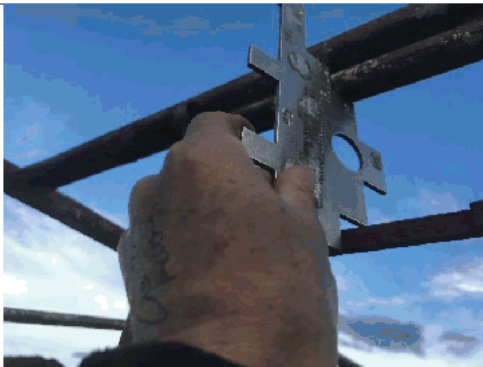
Head entrapment in structure of lullaby swing
