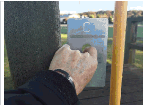
Head entrapment in slide handles (fall over 600mm)
