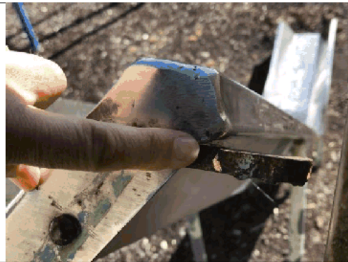
Toggle entrapment at top of slide
