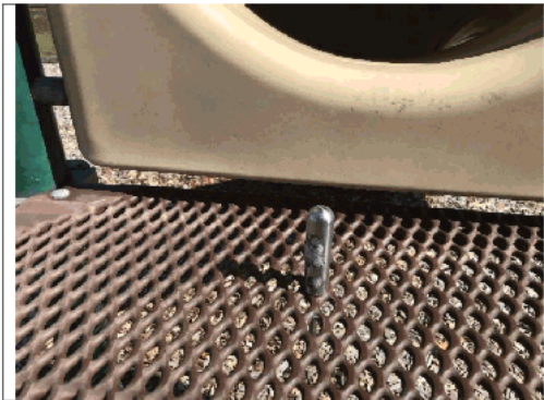
Finger entrapment in deck at slide opening (forced movement)
