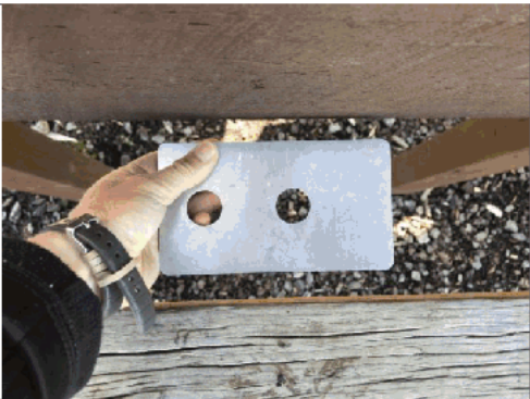
Head entrapment in module between clatter bridge
