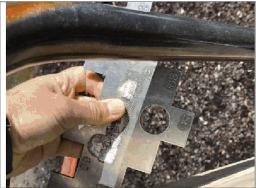
Head entrapment on module
