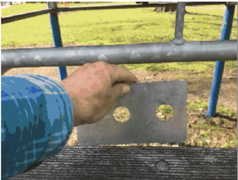
Head entrapment in barrier
