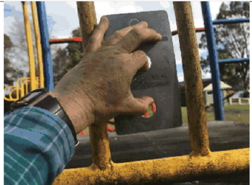
Head entrapment in barrier
