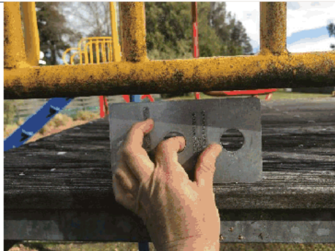
Head entrapment in barrier
