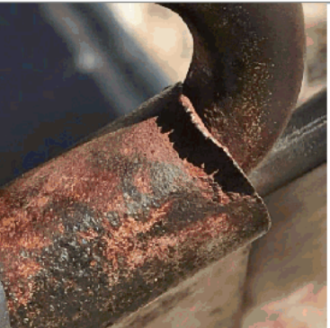
Swing plate burring and sharp
