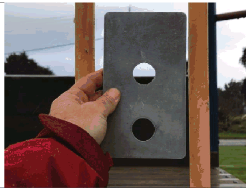
Head entrapment in barrier.
