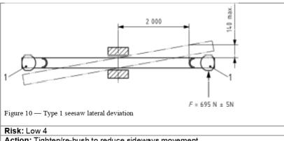
Action: Tighten/re-bush to reduce sideways movement.
