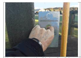
Head entrapment in slide handles (fall over 600mm)
