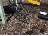
**Standard:** The falling space shall not contain any obstacles onto which a user could fall and cause injuries.
