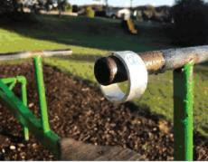
Handles fail ring gauge test (should not pass through ring)
