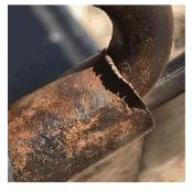
**Standard:** 4.2.5 Finish of Equipment There shall be no protruding nails, projecting wire rope terminations or pointed or sharp-edged components.
