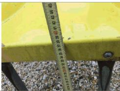
Run out too high on slide – raise loosefill depth to rectify.
