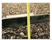
**Standard:** There shall be a ground clearance of at least 400 mm underneath heavy suspended beams,
