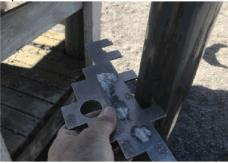
**Standard:** Grip is measured between 16mm and 45mm. The cross section of any support designed to be grasped shall have a width not exceeding 60 mm.
