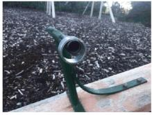
**Standard:** Ring gauge must not pass over the handle or foot rest. NOTE: The intention of this requirement is to reduce the hazard of eye injury from the ends of projecting hand supports, by maintaining a cross sectional area of at least 15 cm<sup>2</sup>.
