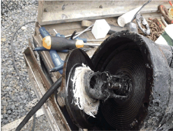
Failed oil seal at Wyndham Waste Water Station due to ragage behind the impellor
