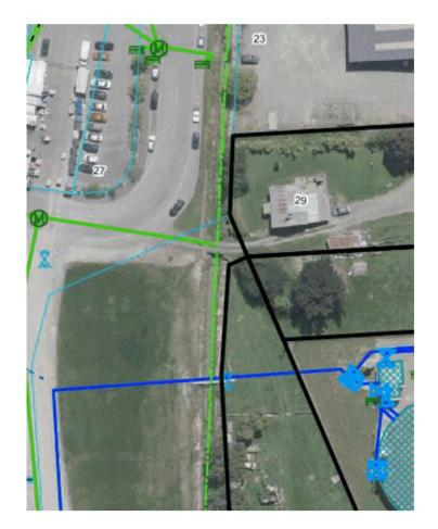
29 Springford Street is identified by black outlines Green lines indicate stormwater (dashed line is an open drain)
