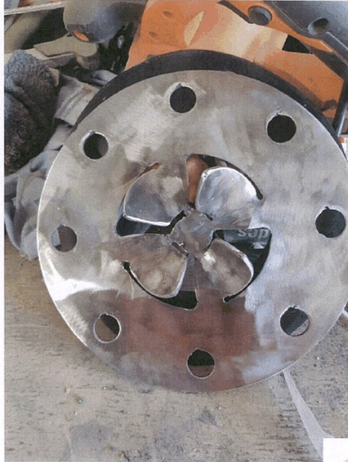
Mixing plate fitted to prevent caustic build up at Otautau WTP
