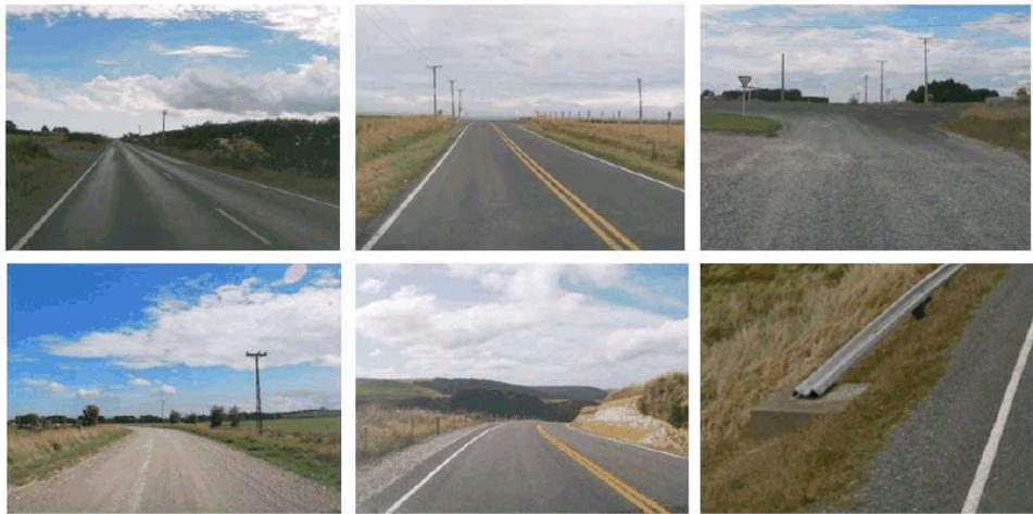
Some of the challenges are (clockwise from top left) high level of carriageway flushing; inconspicuous intersections (e.g. Otautau Nightcaps Road intersection with Hundred Line Road West); gravel migration from unsealed side roads; Texas twist guardrail terminal ends; lack of consistent delineation, particularly on curves; and flat crossfalls on unsealed roads along with inadequate drainage channels.
