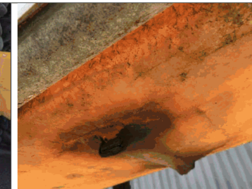
Rust underneath slide
