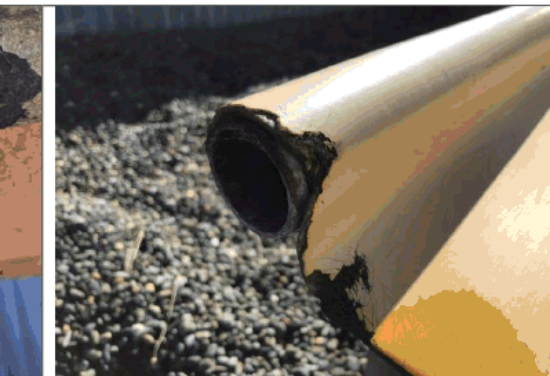
Fibreglass broken, rough at slide end.
