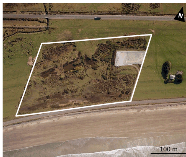
Figure 7 - Former gravel pit site along Colac Foreshore Road showing partial infilling as wetland and landfill. The extracted gravel is thought to have been used to construct the nearby highway visible at the top of the image. White line indicates the approximate gravel pit boundary; white shading indicates approximate landfill extent. Aerial photograph source: SDC, dated 1993.
