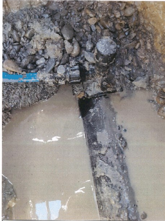
150 PE saddle failure – 31 Prince Street, Winton
