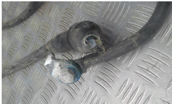
Failed Neutral Cable Elgin Terrace
