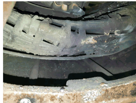
The winding failure on Unit 5 generator
