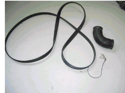
Damaged belt and pipe from Unit 5 failure on 26/1/21
