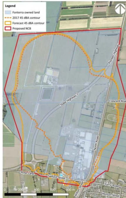
Figure 4 Comparison of proposed NCB and 45dBA contour (Source: MDA Noise Report)
