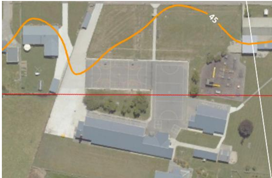
Figure 5: Area 7 updated predicted modelled 45 dB L_{Aeq} noise contour.
